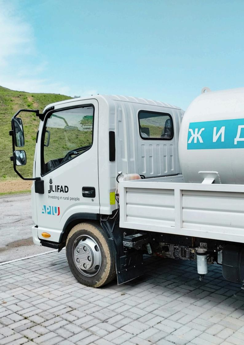
"The Access to Markets project provided the ELITA State Entity with a new 1,600-litre tank truck for transporting nitrogen. This vehicle has already made several trips to the Naryn and Issyk-Kul regions, significantly saving resources: the previous equipment could transport only 1,000 litres." — Irena Baitanaeva, APIU Communication Officer
